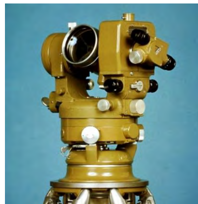
Wild's Double Circle theodolite with Micrometre Kern DKM3 (1939). Accuracy 0.1 sec.
